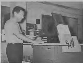
PEDRO YARZAGARAY operates this card reader-punch machine that can read 1000 cards and punch 300 cards a minute.
